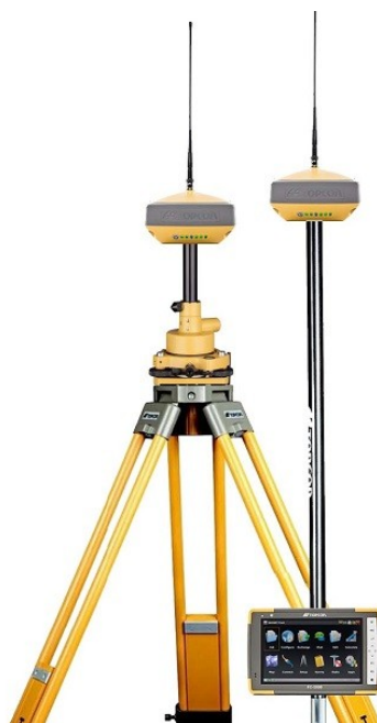
FIGURA 5 - BASE E ROVER TOPCON HIPER VR
